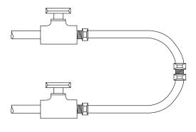
NOTE: Use standard coupling (field-supplied) and hose adapters to join 2 hoses.
